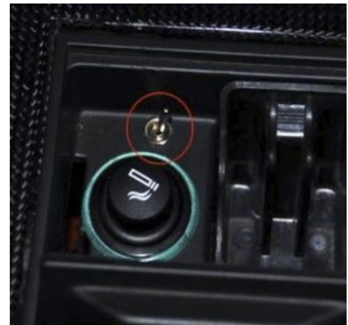
Miniature Toggle Switch mounted in ash tray
